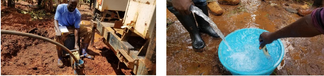
Figure 5: A technician taking results and measuring E.C during test pumping
